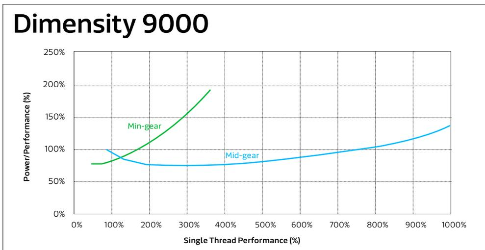
Figure 3.2. Dimensity 9000 CPU power efficiency
