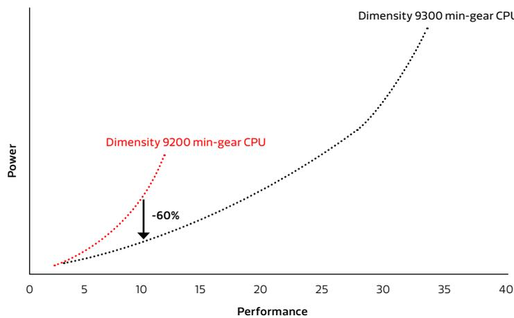
Figure 4.1. Min-gear CPU power efficiency curve comparison between Dimensity 9300 and 9200
