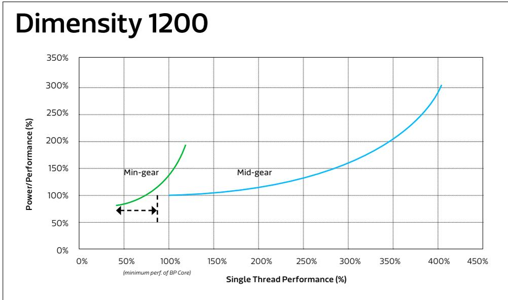
Figure 3.1. Dimensity 1200 CPU power efficiency
